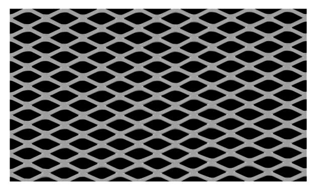
LW Aperture:15.00mmStrand Width:1.80mmSW Aperture:5.30mmThickness:0.90mmWeight:2.90 kg / m2Open Area:62%
